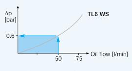
$\Delta T_{\text{oil}} = 33 \text{ x} (12 \text{ kW} / 50 \text{ l/min}) = 7.9 \text{ °C}$
