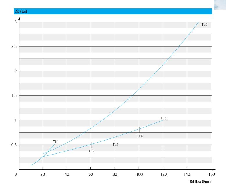
The pressure drop curves are based on a viscosity of 30  $mm^2/s = 30 cSt$ . Please use conversion factor f from page 11, to calculate pressure drop at other viscosity's.
