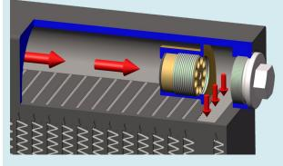
The installation of an external bypass is not necessary reducing costs and mounting space.
